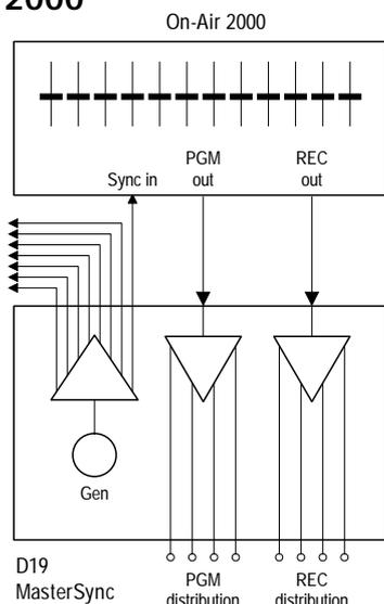
With more and more signals being transported on optical fibre links for improved immunity against signal distortion like hum, many systems have inputs and outputs located remotely. These inputs and outputs must be synchronized to the main digital system.
